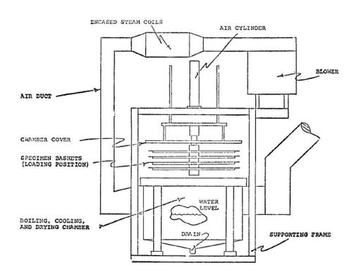
SCATA - accelerated automatized boil test
